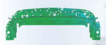
Data generated with the 26 laser line mode. Compared to the CAD file.
