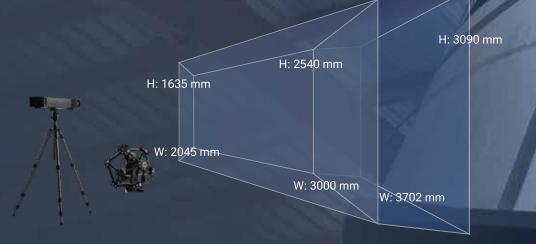
(1) Leapfrog: Refers to the technique of relocating the measuring device to extend its working volume. This involves measuring reference geometries (artifacts) in one position, then repositioning the device and measuring the same reference geometries again. These reference points establish a link between the new device position and the original coordinate system, allowing measurements to be consistently reported in the same reference frame.
